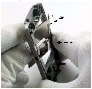
c. Slide the card trap out of the D-cover.
