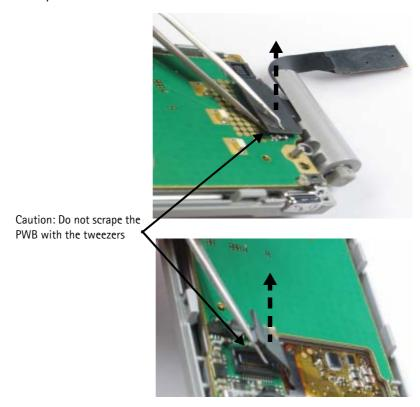
b. Remove the PWB from the A-cover by lifting the bottom of the PWB from the guide pins and sliding the LCD flex cable through the opening.
